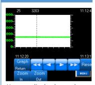
You can display log scales for degree of vacuum (pressure input), and record the data (option).
